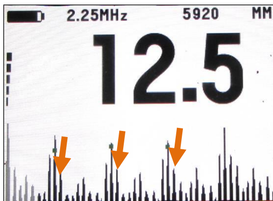
Flat, new steel 12.5mm thick with blind hole (DIVE gauge screenshot).
