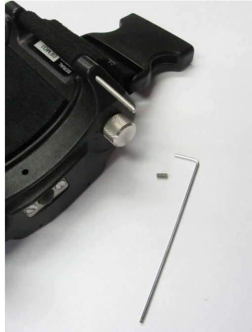
Wrist Strap Pin Securing Grub Screw
