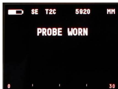
Probe Worn Message on Measurement Screen.
