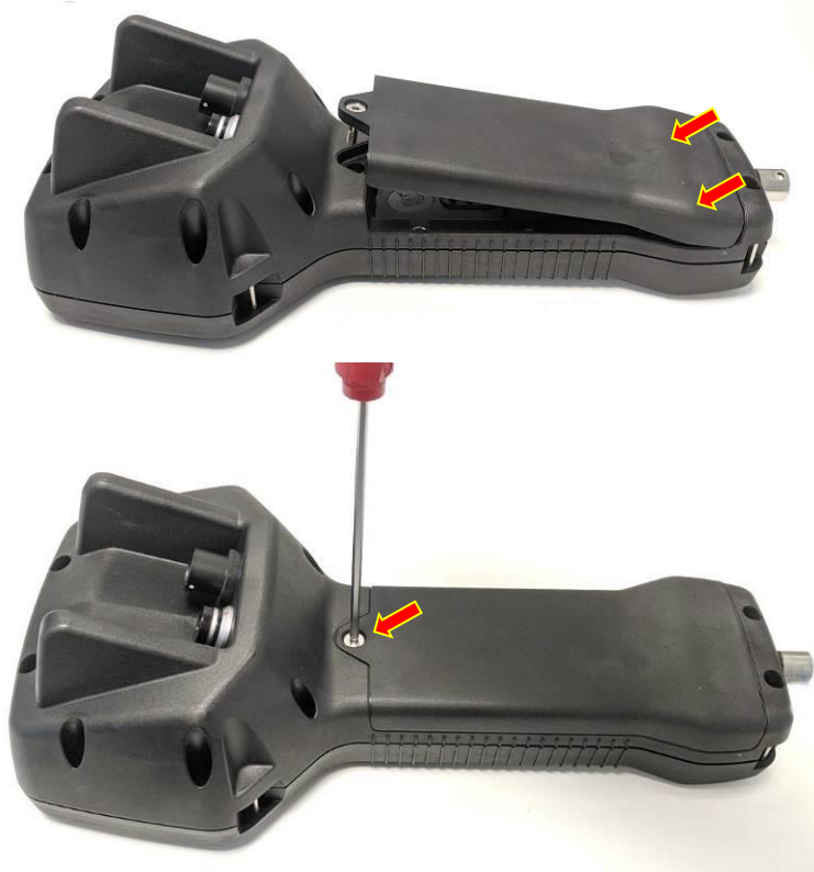
Fig 2. Cygnus 1 Ex Battery Pack Fitting.
