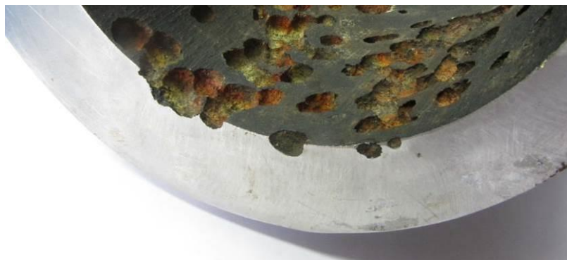
Large Corrosion Pits.
