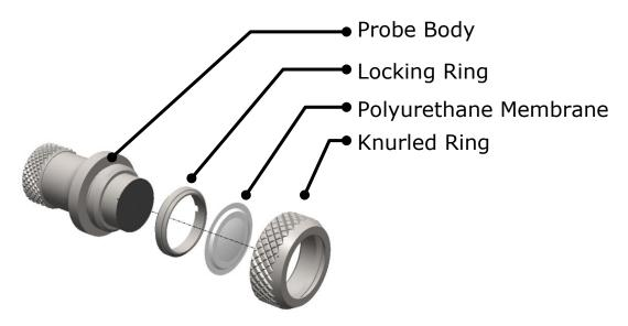
Single Element Probe Membrane Parts.
