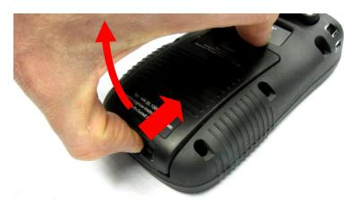
Press the bottom of the battery cover to release the retaining clip and lift up the battery cover.
